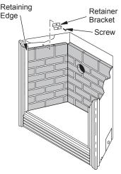
Figure 5 - Securing Side Firebrick Panel to Side Wall of Fireplace
